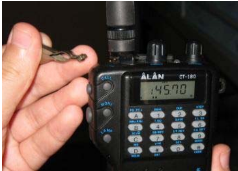
At the pictures you see a hand- held with its “rubber” antenna (100- mm long). The radio is received R4- repiter, which is located 130- km away.
