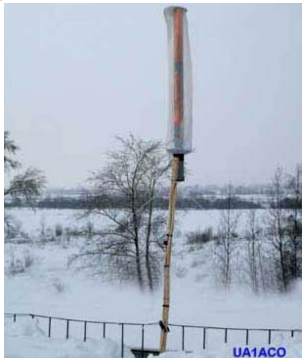
Figure 6 EH- Antenna for the 160- meters on the roof of the house
