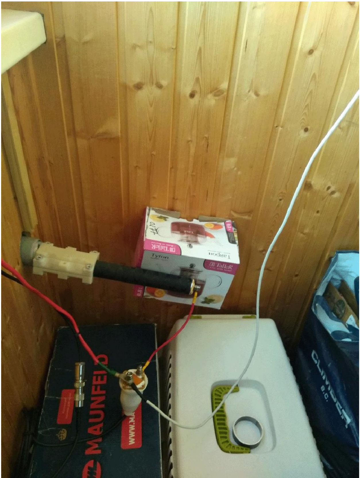
Figure 3 Simple Dipole Antenna for HF Bands Going Inside of the Balcony
