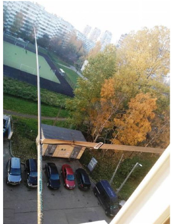
Figure 2 Simple Dipole Antenna for HF Bands on the Wall of the Building
