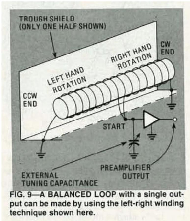
FIG. 9—A BALANCED LOOP with a single output can be made by using the left-right winding technique shown here.
