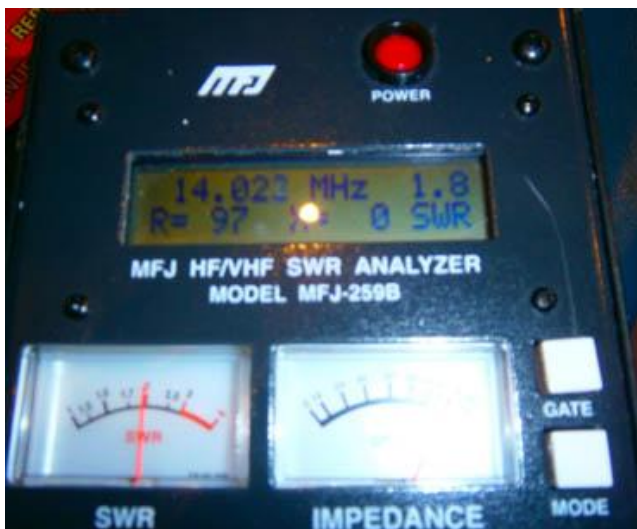
MFJ-259B Shows the Frequency of the Lambda/2 Length
