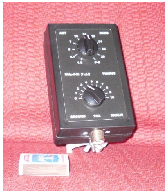
ATU of the Balcony Vertical HF Antenna
