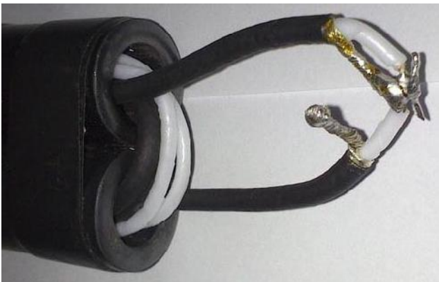
View of the Balun transformer for 50/150 Ohm
