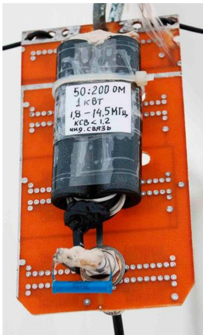
Practical Design of Wide Band Transformer 200/50-Ohm, 1.8- 14.5- MHz with compensation capacitor
