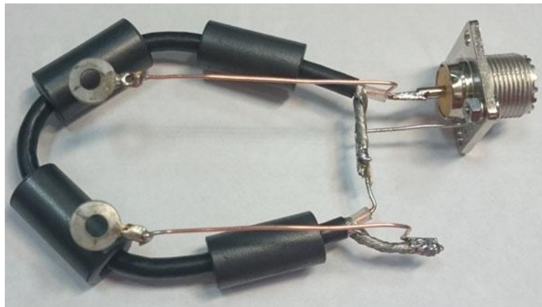
Figure 4 Picture of the Transformer for Balanced Antenna
