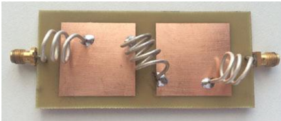
Figure 9 Design of the simple Low Pass Filter for 145 – MHz Band (without internal rejection filters)
