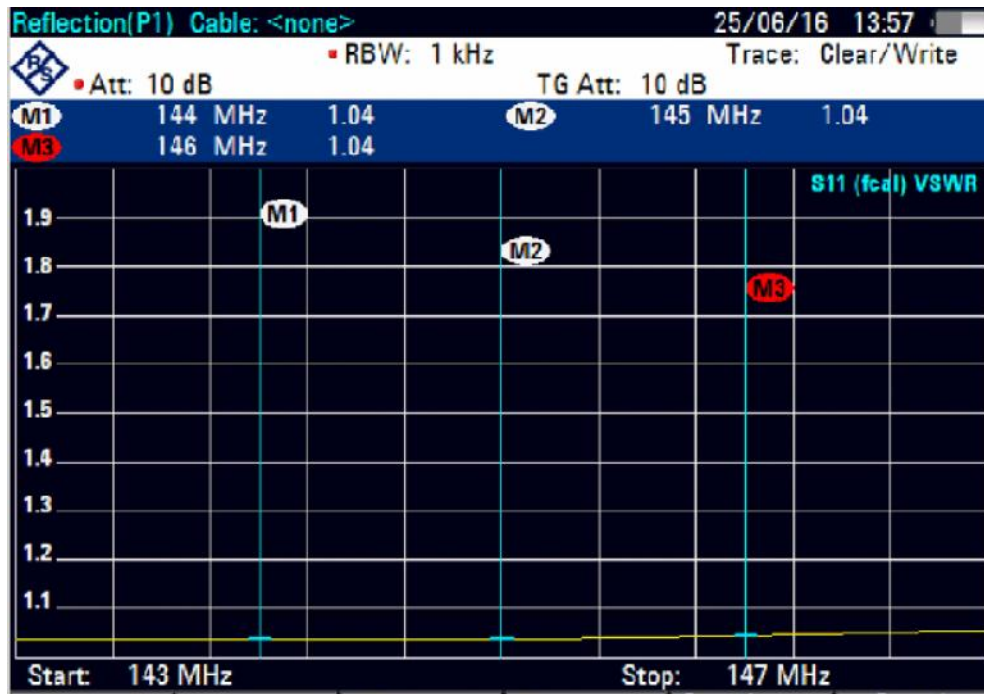
Figure 5 SWR for the Low Pass Filter for 145 – MHz Band at the 2- meter Band
