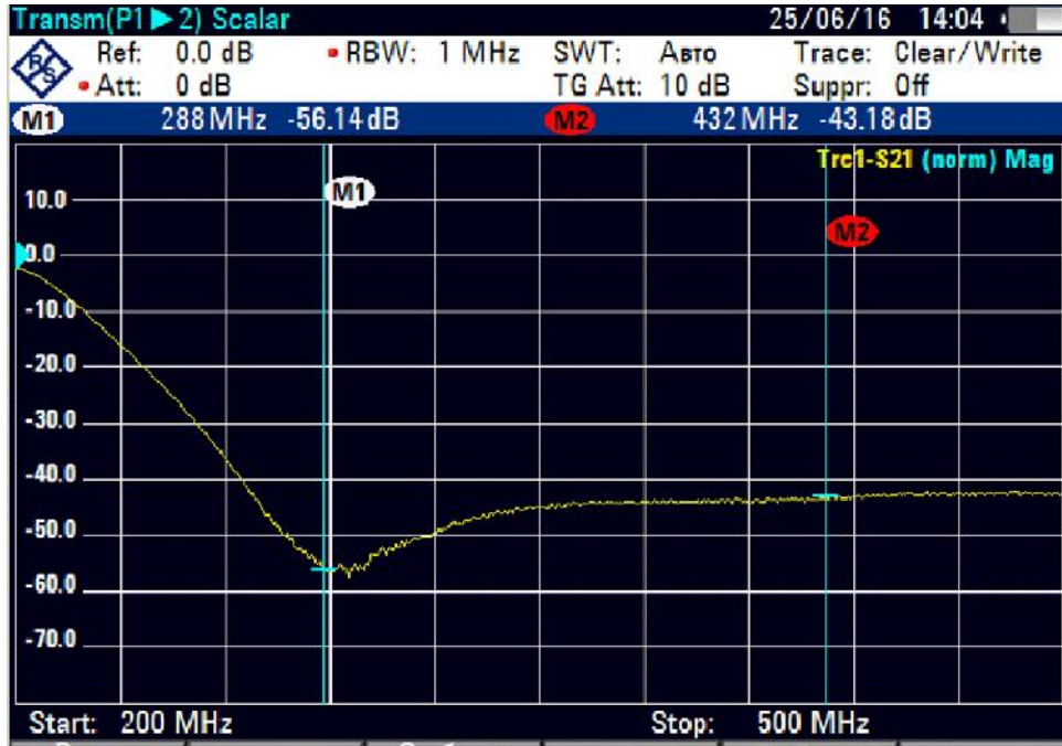
Figure 6 Return losses of the Low Pass Filter for 145 – MHz Band at frequencies 200- 500- MHz
