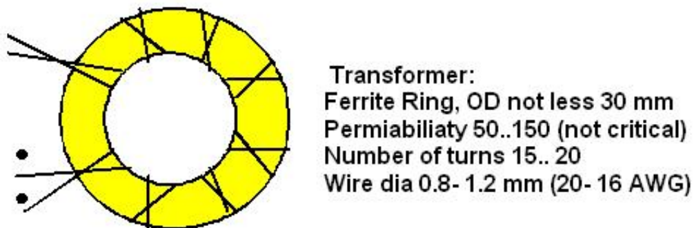
Figure 3 Design of the Balanced Transformer
