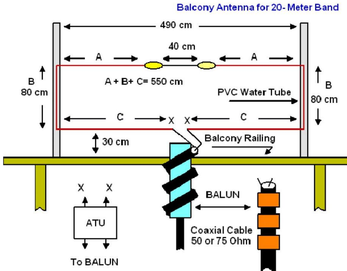
Description and pictures of the Balcony Dipole Antenna for the 20 Meter were published in ham forum at [www.cqham.ru](http://www.cqham.ru). Author of the antenna is unknown to me. However the antenna works and may be used in tight conditions.
