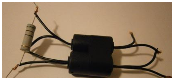
Figure 7 RF Transformer on Two Cylinder Ferrite RF Chokes loaded to 51- Ohm Resistor
