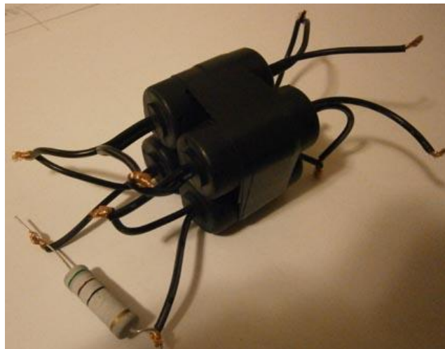
Figure 10 RF Transformer on Four Cylinder Ferrite RF Chokes loaded to 51- Ohm Resistor
