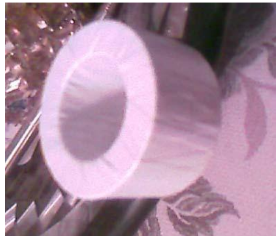
Figure 3 Two Rings Wrapped with Electrical Insulation Tape
