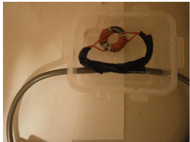
Figure 6 Insulation Transformer Inside Opened Food Box
