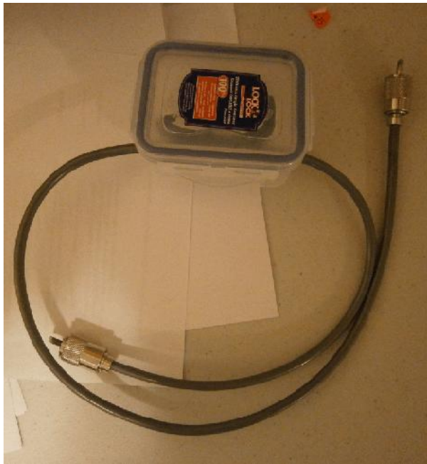
Figure 7 Closed Food Box with Insulation Transformer
