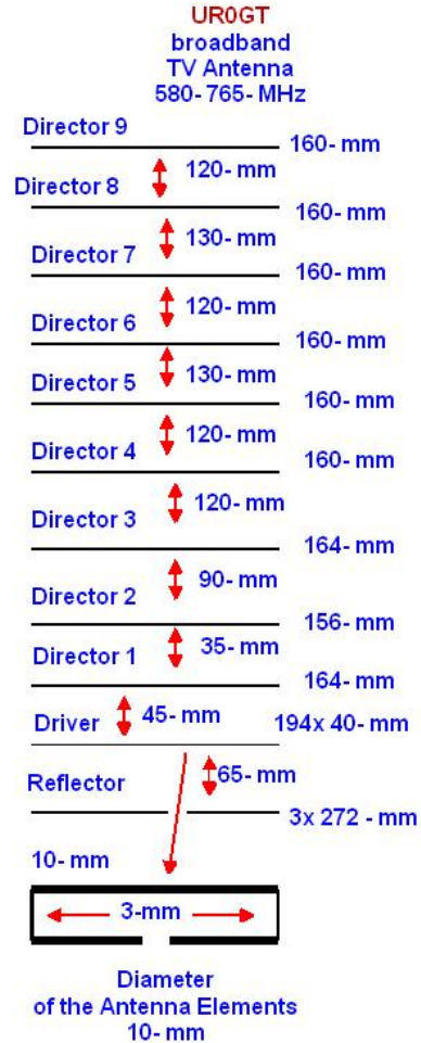
Figure 2 Design of the Broadband TV Antenna
