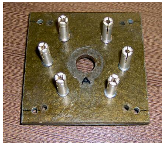
Cylinders were turn on to collet. Tube's pins were polished to smooth inserting into the holders.
