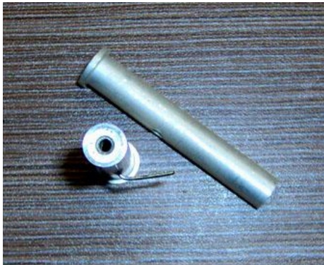
Resonators were removed. Then central hole was drilled to diameter of the tube's pin.
