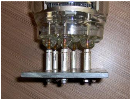
Resonators were removed. Then central hole was drilled to diameter of the tube's pin.
