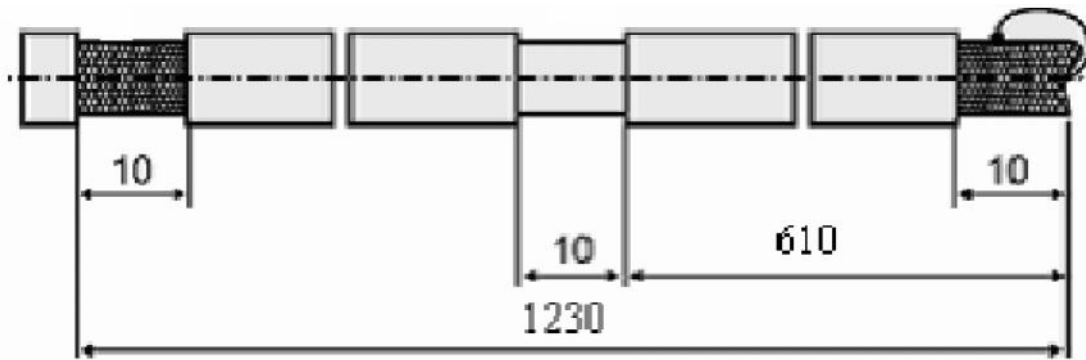
Figure 2 Preparation of the Coupling Loop
