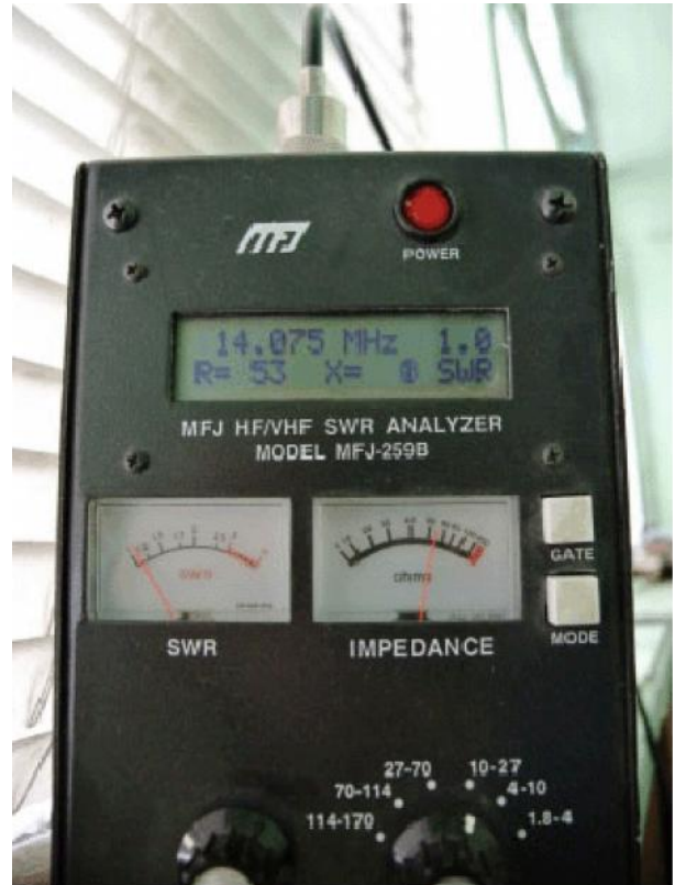
Picture 2 Antenna Analyzer MFJ- 259B Connected to the Tuned into Resonance Antenna
