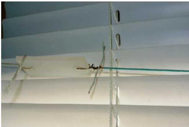
Picture 4 Capacitive Load at the Shortened Dipole Antenna for the 20- meter Band
