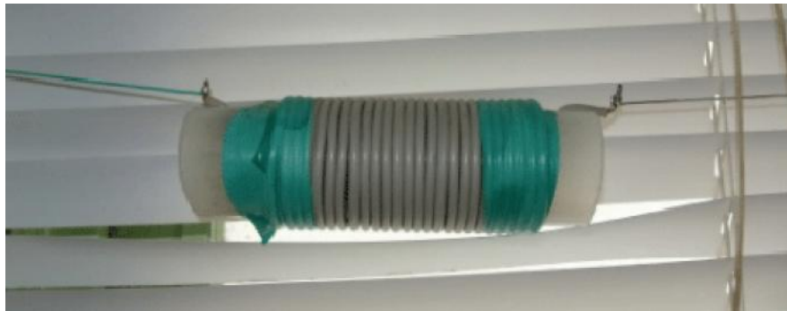
Picture 3 Inductor of the Shortened Dipole Antenna for the 20- meter Band
