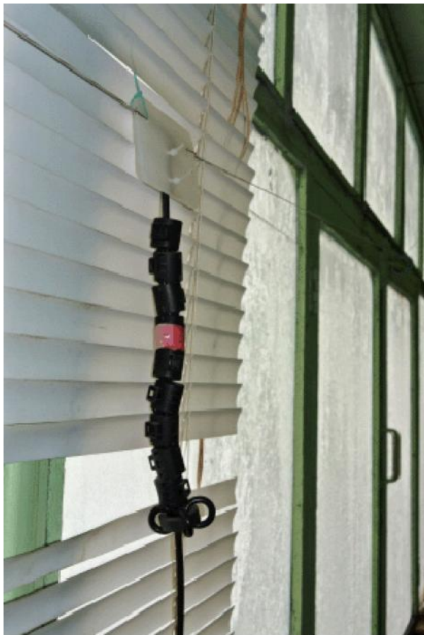
Picture 1 Shortened Dipole Antenna installed at my balcony
