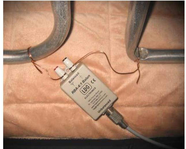
Feed Point of the Lawn Antenna
