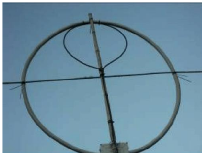
Figure 6 Coupling Loop on the Antenna Loop
