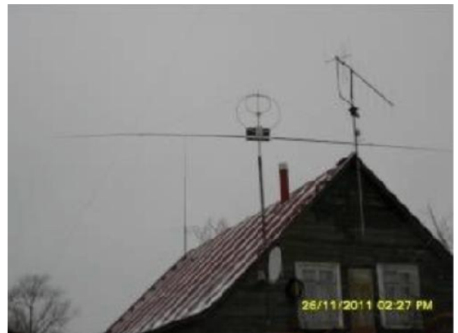
Figure 9 View of the Antenna UA6AGW V.20.0 on a Roof
