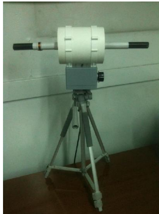
Ferrite Magnetic Antenna for the MW. Ferrite: 3- beams X 7- Ferrite Rods \mu=400 , L= 160- mm, OD- 8- mm.
