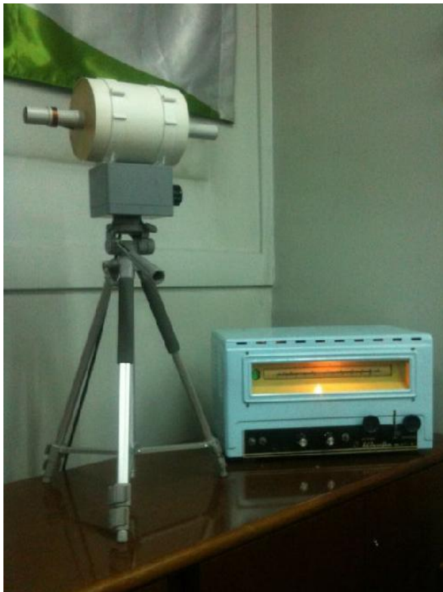
Ferrite Magnetic Antenna for the MW. Ferrite: 2- beams X 7- Ferrite Rods \mu=400 , L= 160- mm, OD- 8- mm.
