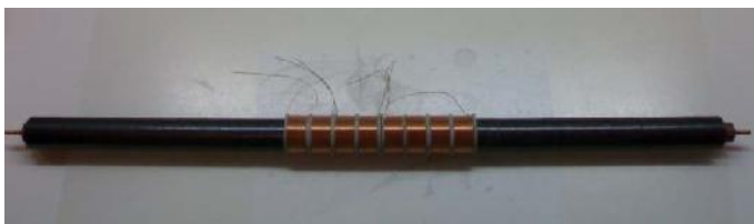
LW Ferrite Antenna. Made of 74 ferrite rings \mu= 2000 , 32 x 20 x 9- mm.
