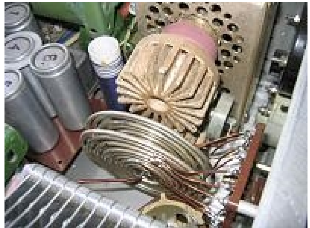
P.A. on GI- 7B. Coiled Inductor Picture by ZLK
