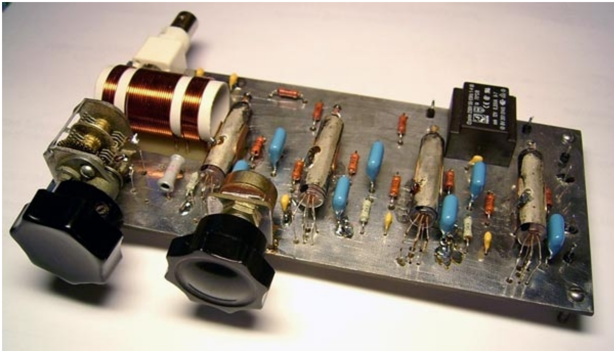
Figure 2 View of the Audion receiver
