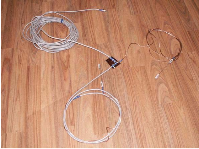
Figure 4 Antenna Strela before installation
