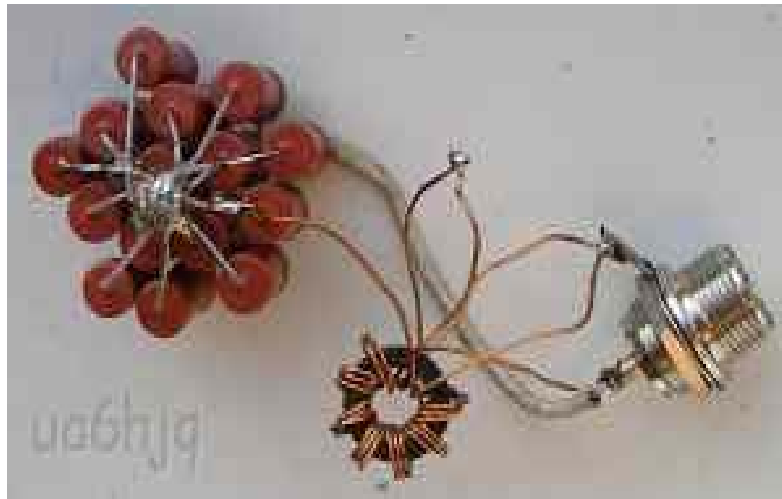
Figure 6 Design of the RF transformer 1:9
