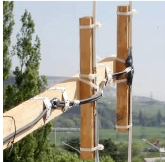
Design of the antenna is very simple. Personally I have made the antenna in 40 minutes. Antenna consists from reflector (length 1002-millimeters) and vibrator (length 972- millimeters, gap for coaxial cable- 10-millimeters). Distance between reflector and vibrator is approximately 204 – 210- millimeters. Antennas parts are made from insulated wire in diameter 4 millimeters. Place of vibrator, where a coax was installed, was protected with a raw compound.
