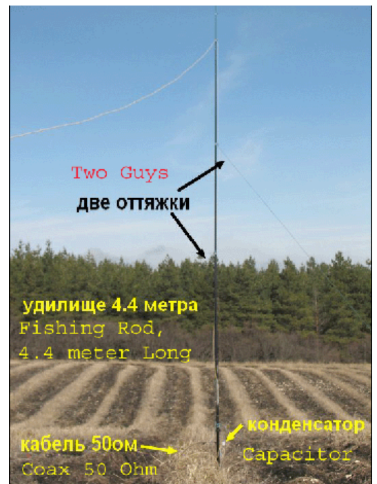
Figure 4 shows the mast of the antenna
