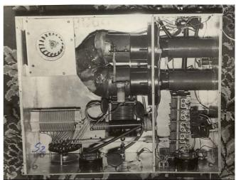
Ventilation: The tubes are blown by the fan (taken from an old tape recorder). Airways are home made- a medical bandage sodden with epoxy. Tubes from medical bandage put on cathodes vent hot air outside the case.
