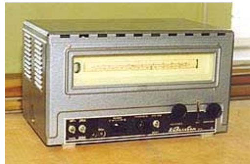
"Kazakhstan". Broadcasting receiver. Model 1963.
