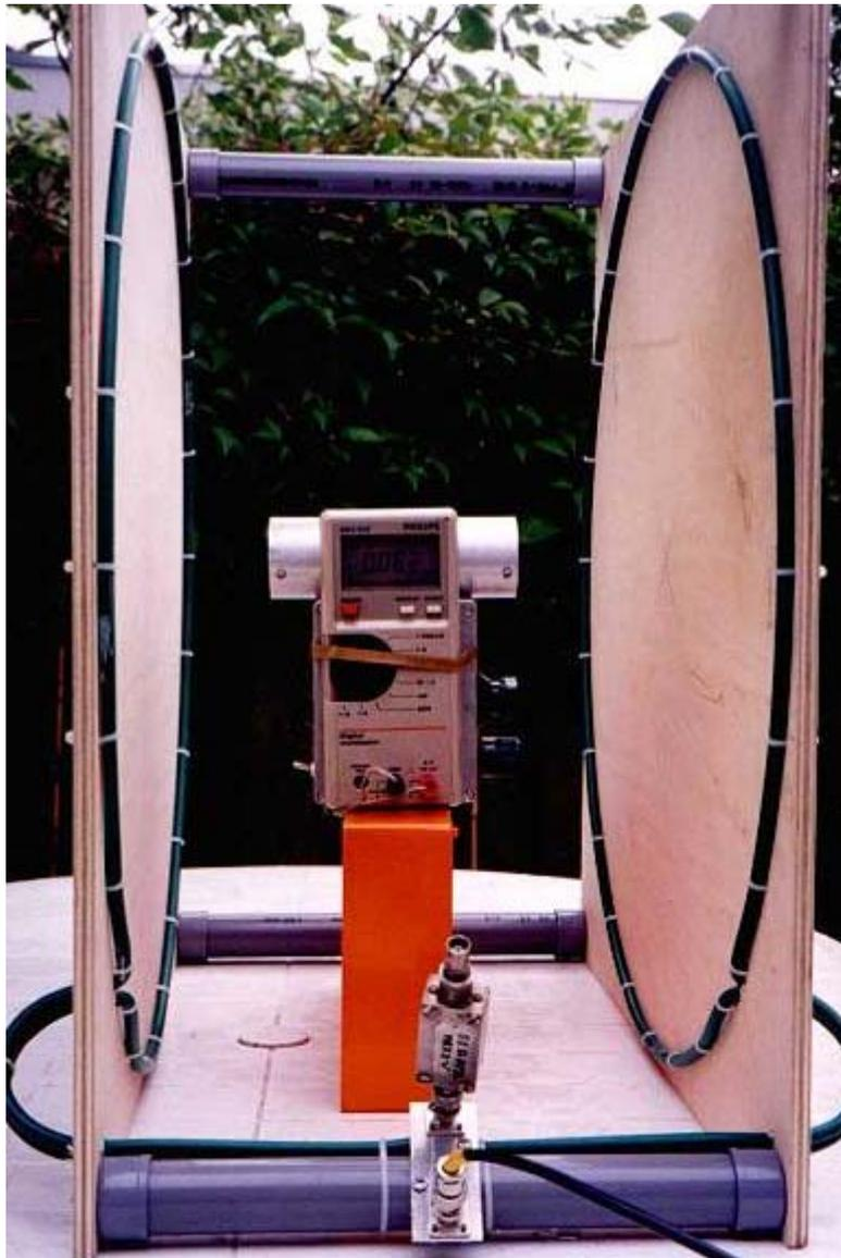
At 137 kHz the reactance of the coils is so low that it can be neglected against the 50 ohm resistor. Therefore when the coil pair in series with 50 ohm is connected to a signal generator with U volt output the current I through the coils in parallel is
